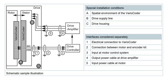
Despite the high electromagnetic immunity, depending on the application, integration into a screening concept may be required for the encoder kit.
